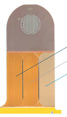
Reduce layers in bend areas by distributing layer routs into segregated sections
