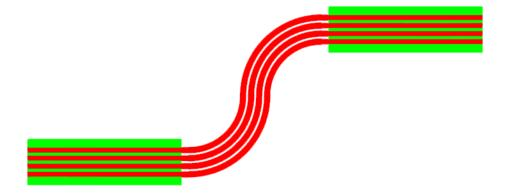
No flex-section stress if rigid boards are horizontally offset- All Flex layers will be same length.
