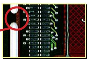
These small holes located at the array tabs work fine to "singulate" rigid boards after assembly but can damage flex parts if the array is twisted or bent to remove the single flex. Unlike rigid boards, rigid flex parts contain flex film layers that will not crack when bent, but could cause delamination. These tabs should be removed by routing or methods other than bending the array.
