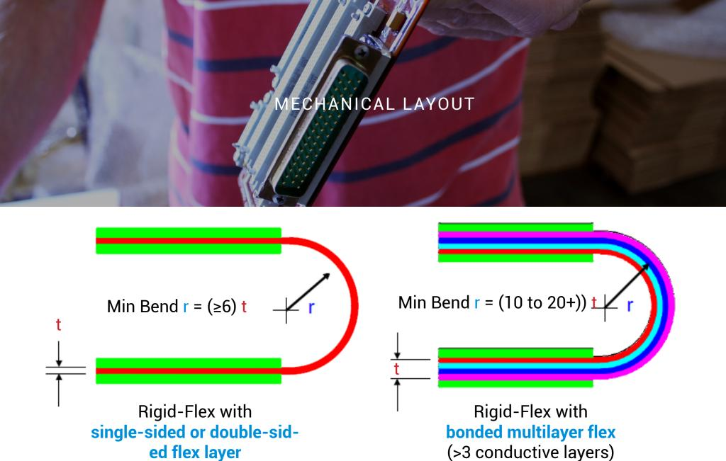
When considering installation and forming: Flex is not sheet metal. Flex is more like a rope.
