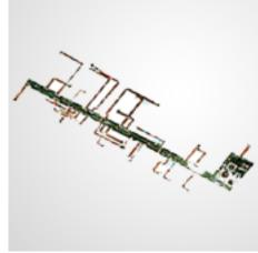
3, 14 LAYER RIGID FLEX NAIL HEAD PIN INTERCONNECT GLOBAL HAWK UAV
