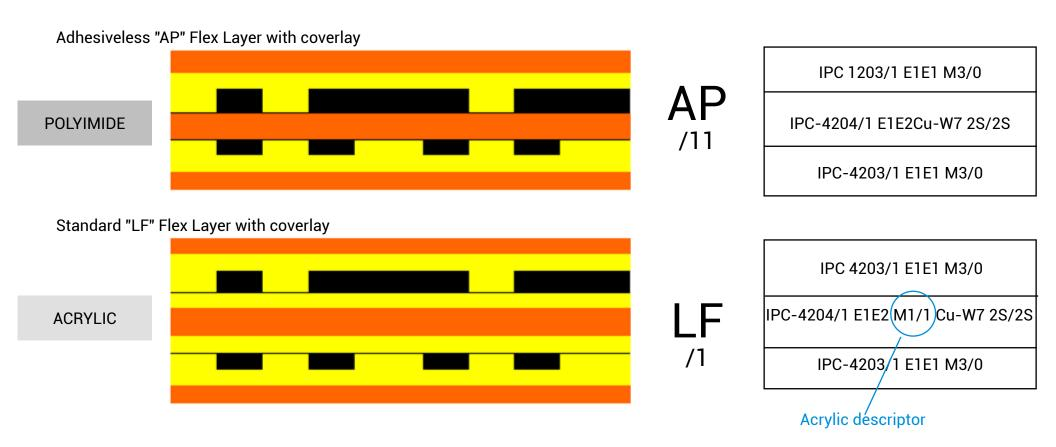
"ADHESIVELESS" simply means acrylic layers are not used to bond to the copper onto the polyimide core dielectric. On adhesiveless constructions, the copper is bonded directly to the polyimide film substrate. AP is DuPont's product code for their adhesiveless polyimide (IPC-4204/11) clad substrates. LF is DuPont's product code for their standard – acrylic / Kapton® (IPC-4204/1) clad substrates.
