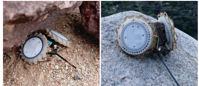
Fig. 11. Latest PUFFER prototype shown folded into a sprawled configuration to fit beneath a rock (left) and climbing a 49° slope (right).
