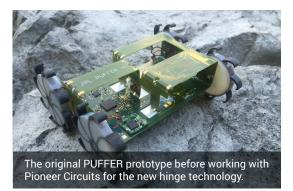
was only able to withstand 1000 test cycles, a very conservative number for a Mars application.
